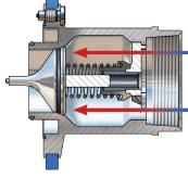
The safety break-away valve consists of two halves, each with a valve that has a o-ring seal.
